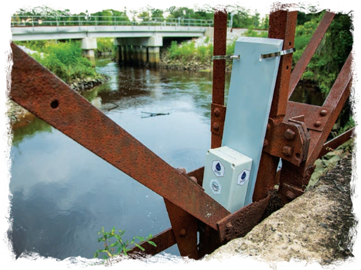
Sea level sensor installed on a bridge in Savannah, Georgia as part of the Smart Sea Level Sensors program.
